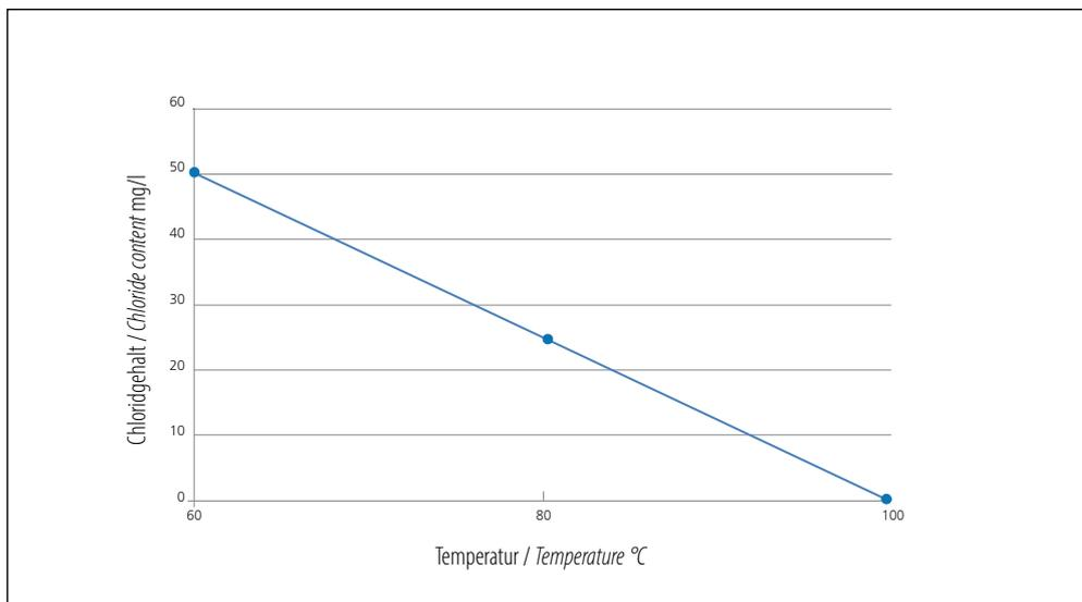
**The main cause of corrosion: chloride ions**
