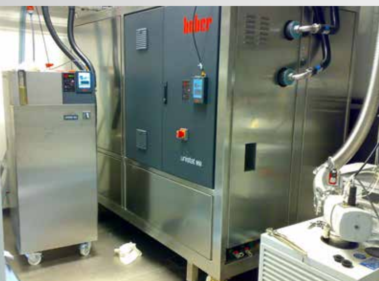
A Unistat 950w controls the temperature in the vacuum chamber, and another Unistat 915w controls the table for the experiments
