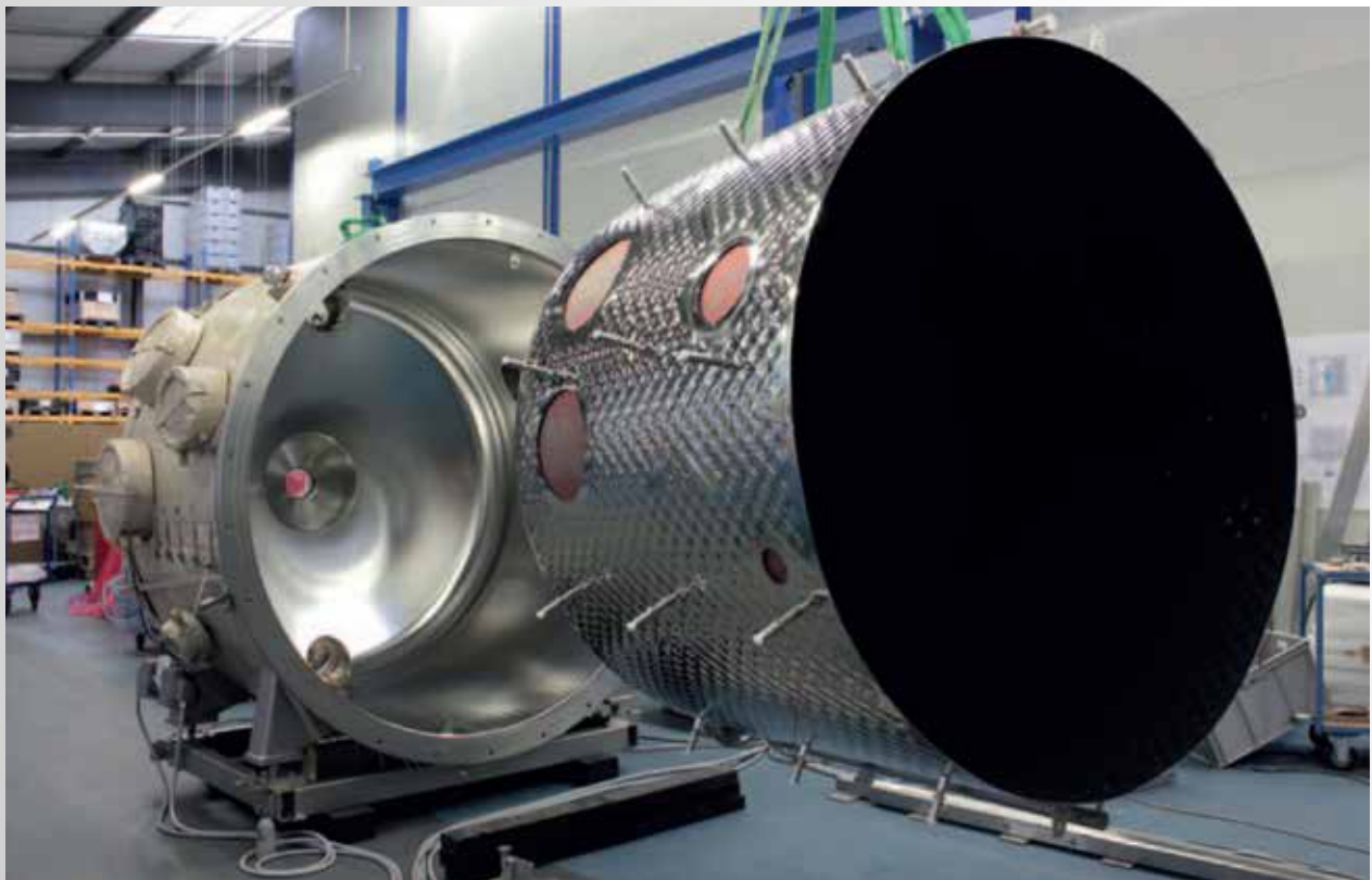
The thermal vacuum chamber is three metres long, with diameter of 1.8 metres. The two halves of the chamber can be easily moved apart and together using a rail system
