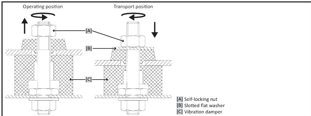
Remove the side panel on the temperature control unit to loosen and tighten the transportation locks.
