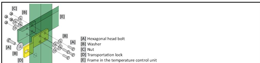
Remove the side panel on the temperature control unit to loosen and tighten the transportation locks.
