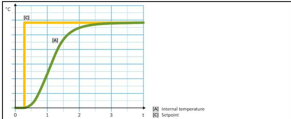
Internal, dynamic temperature control with possible overshooting of the temperature
