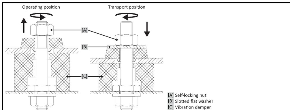
Remove the side panel on the temperature control unit to loosen and tighten the transportation locks.
