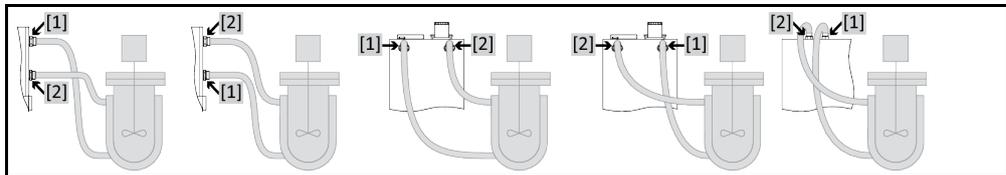
To enable your application to be operated correctly and eliminate air bubbles from the system, you must ensure that the >Circulation flow< [1] connection from the temperature control unit is attached to the lower connection point of the application and the >Circulation return< [2] into the temperature control unit is attached to the higher connection point of the application.
