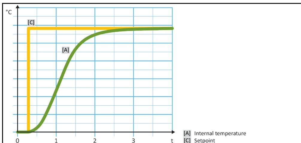
Internal, dynamic temperature control with possible overshooting of the temperature
