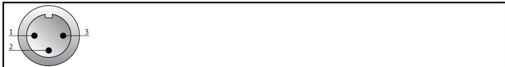
The connection is designed as a potential-free changeover contact.
