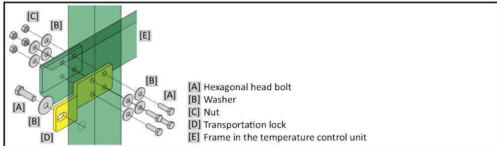
Remove the side panel on the temperature control unit to loosen and tighten the transportation locks.
