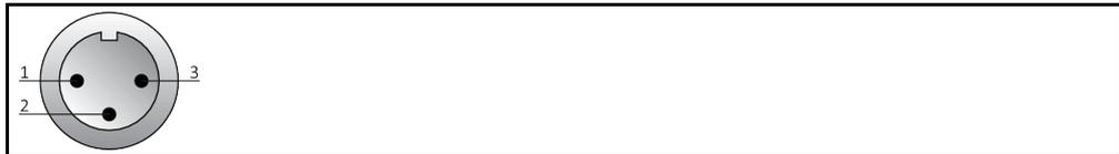
The connection is designed as a floating changeover contact.
