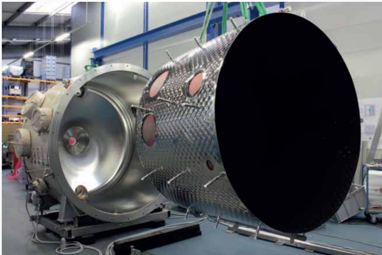
The thermal vacuum chamber is three metres long and has a diameter of 1.8 metres. The two halves of the chamber can be easily pulled apart and pushed together using a rail system.
