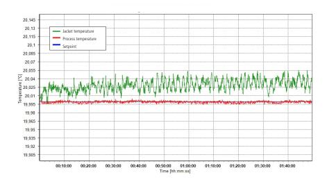
The graphic below shows the stability of the process mass at +150°C is +/-0.03K
