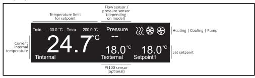
Home screen: Temperature control is inactive or an error message is displayed
