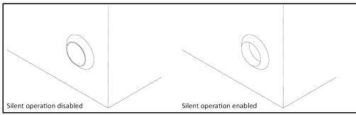
Enabling silent operation on the temperature control unit reduces the noise level by decreasing the pump capacity. For the exact position of the switch >Change pump speed< [114] please refer to the "Wiring diagram". → From page 69, section »Annex«.
