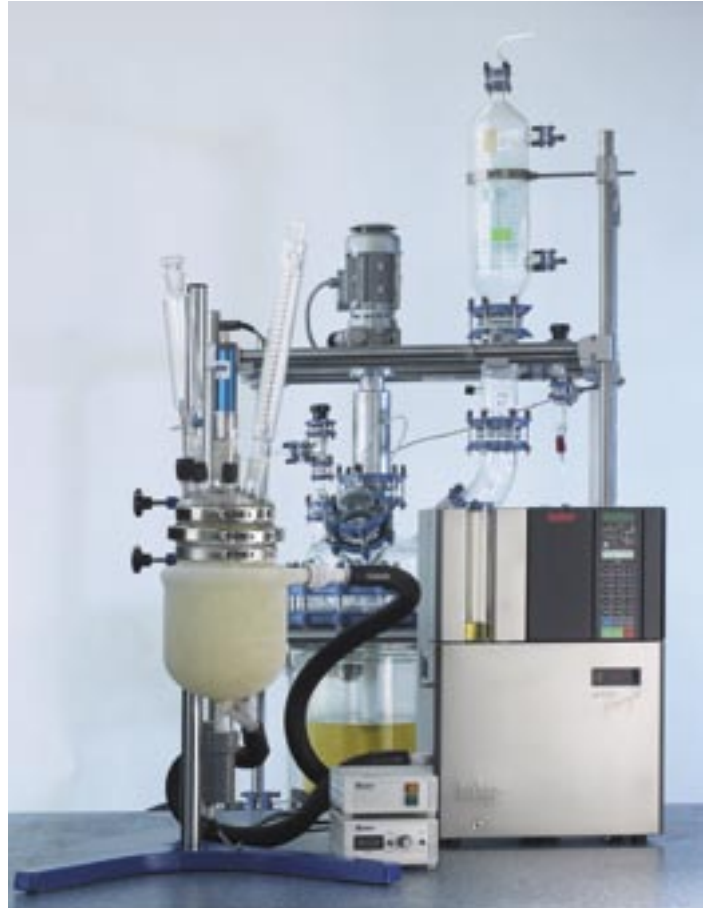
Unistat Tango connected to the Buddeberg 2-litre reactor
